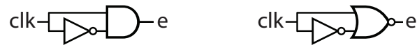
Figure 1.2: Edge detect circuits that limit the JK flip flop to flip states only once during each clock pulse, during (left) the rising edge of each pulse, or (right) the falling edge of each pulse.
