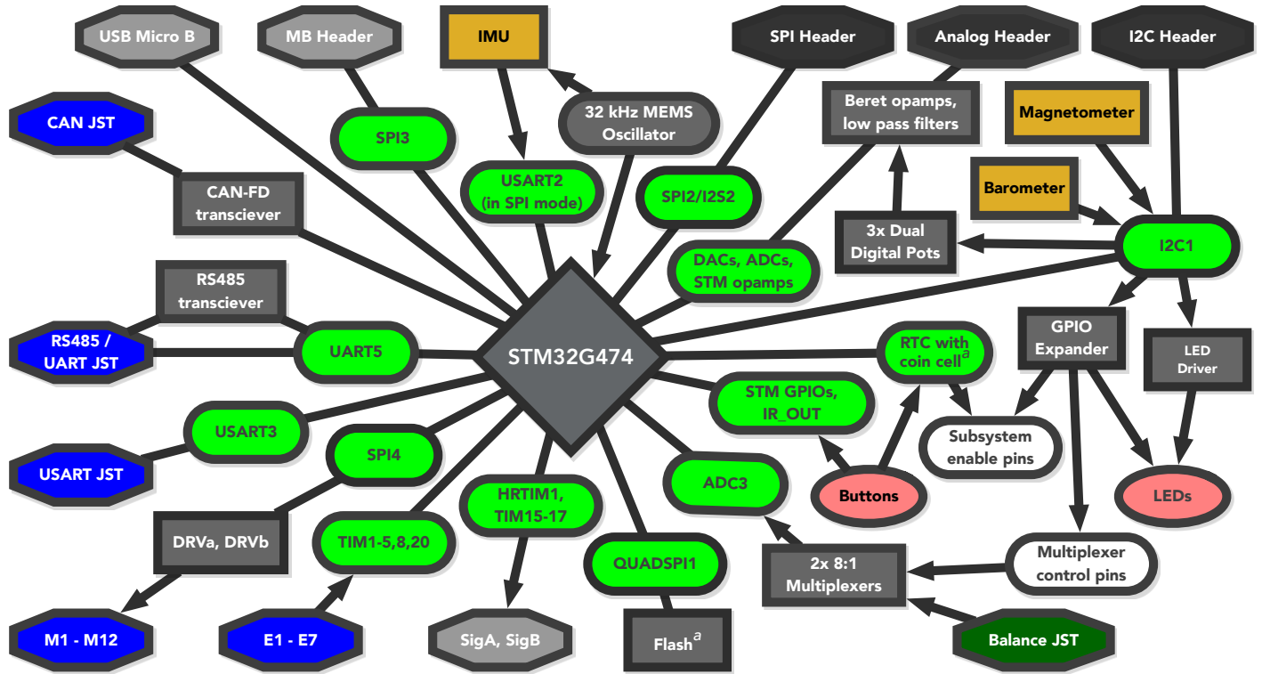
Figure 5.9: Connectivity of the primary STM buses on Berets, with rectangles denoting ICs, brown rectangles denoting environmental sensors, octagons denoting connectors, capsules denoting channels, ellipses denoting buttons & LEDs, and () a denoting optional backside components. See Table 5.4 for the correspondence between Beret channel names and the STM32 hardware channel names.
