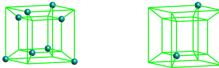
Figure 12.2: Codewords of (left) the (SED) [4, 3, 2] LBC; (right) its dual, the (quasi-perfect, SECDED) [4, 1, 4] LBC.
