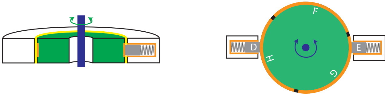
Figure 3.2: Brush & commutator systems for transferring both DC and AC power and signals between rotating (green) and non-rotating parts. (a) Side (cut-away) view of a continuous-ring brush/commutator system ; a spring is used to keep the (relatively soft) carbon graphite brush (gray), which is stationary, in constant contact with the copper commutator (orange) mounted to the rotating component (green) attached to the shaft (blue). (b) Top view of split-ring brush/commutator system for coordinated excitation of the rotating electromagnets of a BDC motor, with brushes {D,E} and commutators {F,G,H} labelled as in Figure 3.9. Images are schematic representations only; for notational clarity, the housings and bearings that keep the parts aligned and spinning freely are not shown.
