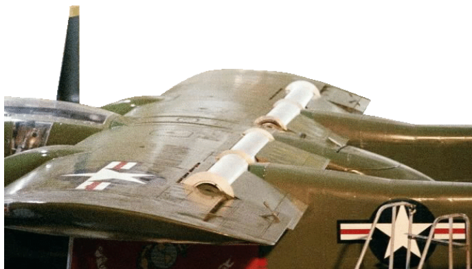
Figure 4: Follow-on tests to those in Peru were performed at NASA-Ames on this modified OV-10A, using essentially the same design (Cichy, Harris, & MacKay [4]). Note that the gap between the cylinder and the wing surface is extremely narrow in this implementation. Photographs by the author.
