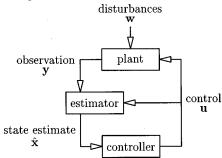
The plant, forced by external disturbances, has an internal state  $\mathbf{x}$  which cannot be observed. Instead, a noisy observation  $\mathbf{y}$  is made and an estimate of the state  $\hat{\mathbf{x}}$  determined. This state estimate is then fed through the controller to determine the control  $\mathbf{u}$  to be applied on the plant to regulate  $\mathbf{x}$  to zero.
