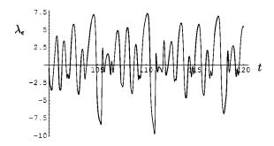
FIG. 4. The local Lyapunov exponent  $\lambda_{\epsilon}(t)$  for the uncontrolled system (as computed with the Euclidean norm) as the state moves on the attractor. The average of the local Lyapunov exponent integrated over the path of the attractor gives the Lyapunov exponent  $\lambda_{\infty}$ =0.707, indicating that perturbed trajectories diverge exponentially.
