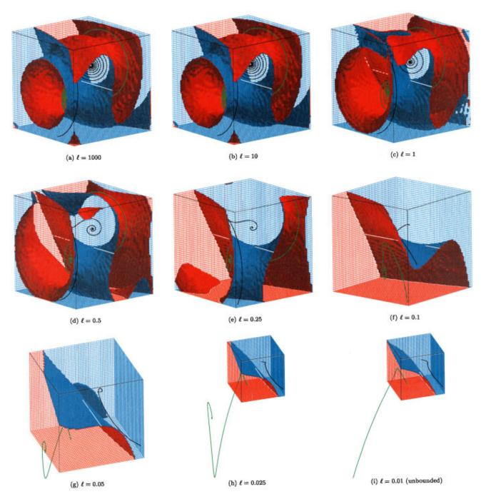
FIG. 5. Regions of attraction of desired (blue) and undesired (red) stationary points in linearly controlled convection system and typical trajectories in each region (black and green, respectively). The cubical domain illustrated is  $\Omega = (-25,25)^3$  in all nine subfigures; for clarity, slightly different viewpoints are used in each subfigure.
