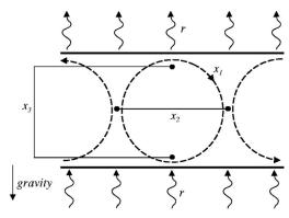
(a) Semi-infinite 2D convection rollers.
