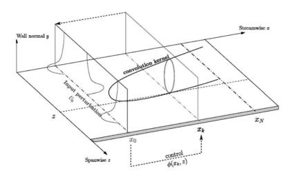
Fig. 3. Relation between the flow system and the control input. The control  $\phi$  ( $x = x_k, z$ ) is found by convolving the feedback kernel  $K^0$  in the plane  $x = x_k$  with the augmented state  $\mathbf{q}_0^a$  in the vicinity of the spanwise location z.
