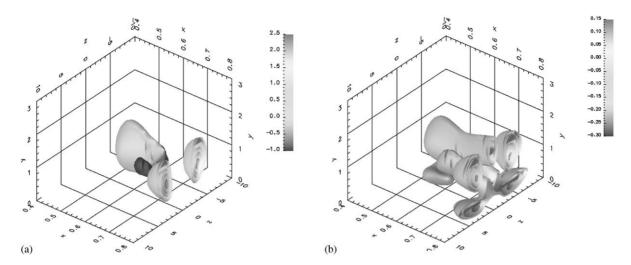
Fig. 4. Isosurfaces of the components of the feedback convolution kernels  $K^0(x, y, z)$  relating (a) the streamwise component of the velocity u (x = 0.5, y, z) and (b) the wall-normal component of the velocity v (x = 0.5, y, z) to the control input  $\phi$  (x, z = 0) on  $x \in [0.5, 0.8]$ . The cost function in this case is the minimization of the perturbation energy at x = 0.8.
