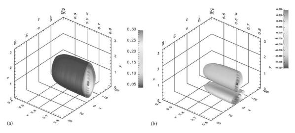
Fig. 2. Isosurfaces of the components of the feedback convolution kernel  $K^0(x, y, z)$  relating (a) the streamwise component of the velocity u (x = 0.5, y, z) and (b) the wall-normal component of the velocity v (x = 0.5, y, z) to the control input  $\phi$  (x, z = 0) on  $x \in [0.5, 0.8]$ . The cost function in this case is the minimization of the perturbation energy on the interval  $x \in [0.5, 0.8]$ .
