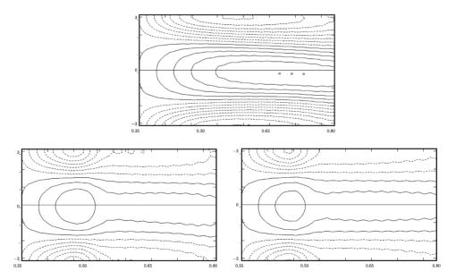
Fig. 5. Longitudinal streaks without control (top), with present feedback control strategy (bottom left), and with the iterative adjoint-based control optimisation strategy of [5] (bottom right).
