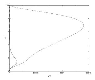
Fig. 1. Control gain for  $\beta$ =0.1 related to the normal vorticity, at the middle of the control domain [0.5, 0.8], using (—) a wall-weighted objective function, and (- - -) an objective function without a wall-weighting term.
