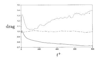
FIG. 1. Drag evolution for the uncontrolled case (dot-dash), detection plane at  $y^+ \approx 15$  case (solid), and control detection plane at  $y^+ \approx 25$  case (dash).
