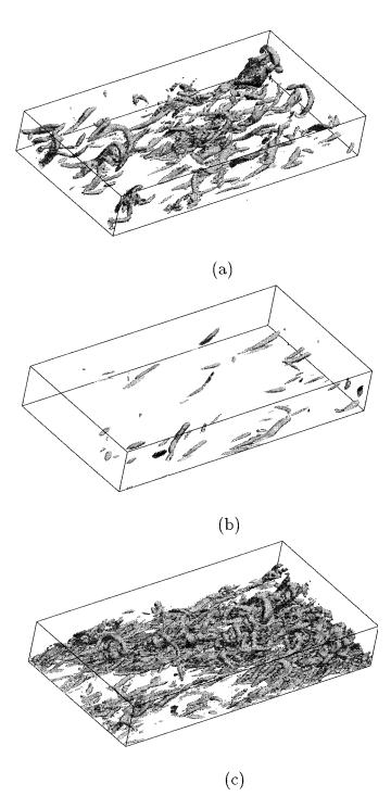
FIG. 2. Isosurfaces of the discriminant of the velocity gradient tensor for (a) uncontrolled baseline case; (b) detection at  $y^+ \approx 15$  scheme at  $t^+ \approx 280$ ; (c) detection at  $y^+ \approx 25$  scheme, also at  $t^+ \approx 280$ . For clarity, only one-quarter of the lower half of the computational domain is shown. Flow is from left to right; the same value of the discriminant was used for (a)–(c).
