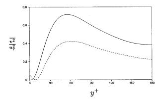
FIG. 3. Turbulent intensities in the wall-normal direction averaged over time and x and z directions. The solid line is for the baseline uncontrolled case, and the dashed line represents the control scheme based on detection at  $y^+ \approx 15$ . The peak magnitudes of  $\overline{u^2}$  and  $\overline{w^2}$  are reduced by the control by a similar proportion to the reduction of peak magnitude of  $v^2$  shown here.
