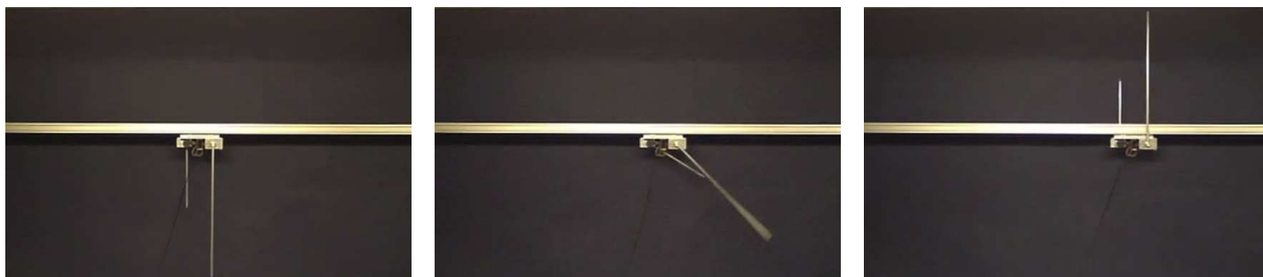
Figure 9: The reference double inverted pendulum swing-up and stabilization problem.
