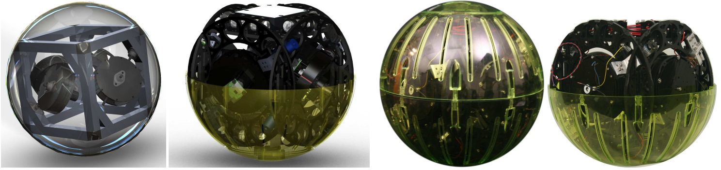
Figure 6: The iceCube concept (a), completed CAD design (b), and prototype (c,d). The hundreds of complex pieces that comprise iceCube fit together with extremely tight clearances; its design would have been impossible without an accurate CAD model.
