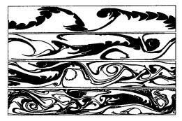
Figure 5: Dye distribution for controlled flow at t = 55, 65, 75 and 85 (from top towards bottom).
