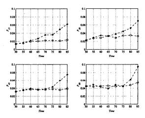
Figure 7: Probability of well mixedness for the uncontrolled case (o) and controlled case (\*).
