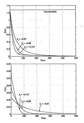
Figure 2: Energy  $E(\mathbf{w})$  and control effort  $C(\mathbf{w})$  for wall-normal, stabilizing control.
