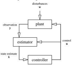
The plant, forced by external disturbances, has an internal state  $\mathbf{x}$
