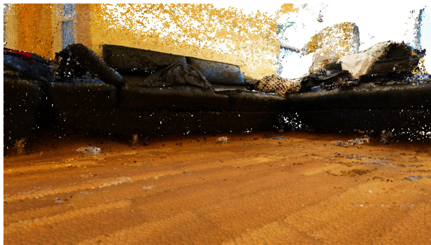
Fig. 13 Point cloud-based 3D map generated using SLAM on BeagleRover.
