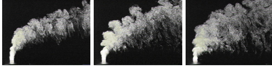
Figure 1.4. Flow visualization from experiments of instantaneous scalar concentration in an x-y plane through the jet centerline for the unforced jet in crossflow (left) and the jet in crossflow forced at St_d = 0.08 (center) and St_d = 0.1875 (right)
