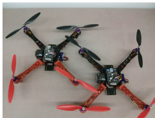
Figure 3. BeagleQuad, a reference aerial platform for studying 3D dynamics, autopilots, attitude hold, and multivehicle coordination. BeagleMiP, BeagleRover, and BeagleQuad share the same electronics and codebase.
