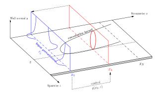
Fig. 2. Relation between the convolution control kernel and the control. The control  $\phi(x=x_k,z)$  is found by convolving the convolution kernel  $K^0$  in the plane  $x=x_k$  with the augmented state  $\mathbf{q}_0^a$  in the vicinity of the spanwise location z.
