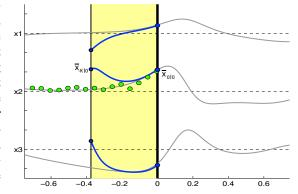
Figure 2. To determine the accuracy of the current estimate (that is, its correlation with the recent measurements), the ensemble at the current time is marched backwards using the system equations until the trajectory of the ensemble mean is significantly divergent from the observations. This gives the current best estimate at the past time,  $\bar{\mathbf{x}}_{-K|0}$ .
