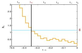
Figure 3. The accumulation of "bias" between the estimate trajectory and the observations is shown as the original estimate is marched backwards. Upon reaching a critical bias  $\bar{B}$ , the retrograde march is stopped. This time  $t_{-K}$  defines the width of the subsequent variational window.
