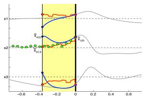
Figure 4. In order to fully define the variational cost function, the background terms at  $t_{-K}$  must be recalled. This is done by marching the original ensemble  $\widehat{\mathbf{X}}_{0|0}$  backwards through the window, sequentially removing the effect of each measurement. This march results in a background ensemble  $\widehat{\mathbf{X}}_{-K|-K}$  at the left edge of the window of interest. From this ensemble, the background mean and covariance can be inferred.
