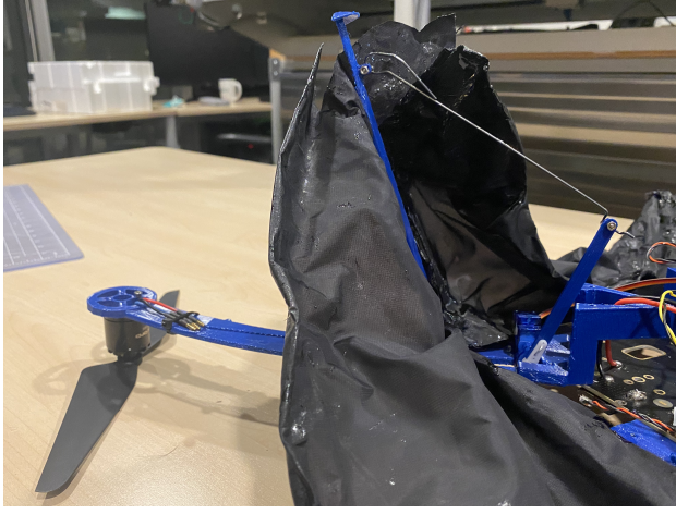
(a) Demo of 4-bar linkage on a rotor arm.
