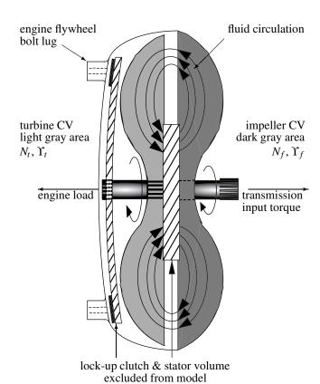
Figure 1: Cross-section schematic of a torque converter
