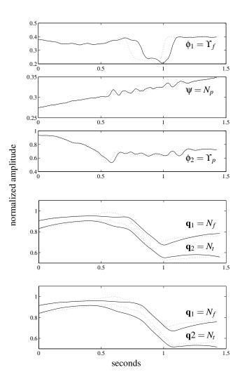
**Figure 2:** Inputs and outputs for the generally identified torque converter model with 18 parameters
