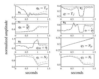
**Figure 5:** States and outputs from the identified model in (3) and (4) given the inputs from figure 4 compared to the performance objectives and the experiment
