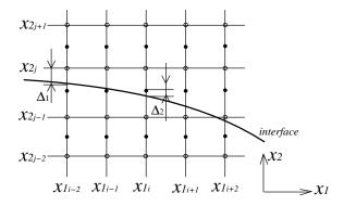
Figure 5. Diagram of the deformed wall and the staggered grid
