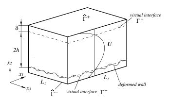
Figure 4. Diagram of the computational domain
