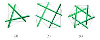
**Figure 1.** Stable tensegrity unit cells. (a) Three-bar cell, (b) four-bar cell, and (c) six-bar cell.
