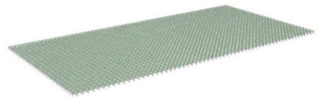
**Figure 2**. A tensegrity fabric with a membrane stretched over the top.
