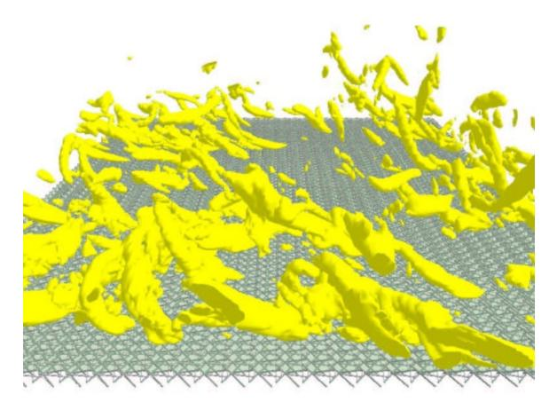
**Figure 10.** A simulation of the mutual interaction of a turbulent flow and a compliant tensegrity fabric separated by a flexible membrane attached to the top nodes of the tensegrity fabric. The viewpoint is from upstream and slightly above the wall; the flow direction is into the page. See <a href="http://turbulence.ucsd.edu/gallery/tensegrity.html">http://turbulence.ucsd.edu/gallery/tensegrity.html</a> for an animation of this result.
