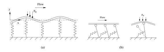
Figure 3. Spring-supported compliant wall models. (a) Isotropic model, (b) anisotropic model. (Adapted from Carpenter *et al.*, 1985, 1990).
