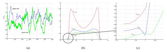
Figure 7. Statistics for deforming wall opposition control using the immersed boundary method. (a) History of drag; (b) profiles of RMS velocity fluctuations; (c) zoom-in view of the lower wall region in (b).
