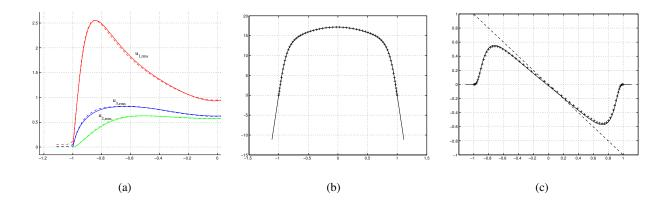
**Figure 6.** Comparison of selected time-averaged statistics from simulations of the immersed boundary method and the regular domain. (a) Profiles of RMS velocity fluctuations; (b) mean velocity profiles; (c) profiles of Reynolds stress and total stress. Solid ——, simulation from the immersed boundary method; dashed (---) in (a) and plus sign (+) in (b) and (c), simulation from the regular domain.
