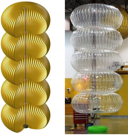
Figure 1: Constant-mass buoyancy-controlled balloon design developed by Thin Red Line (see [4], [5]).
