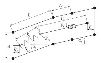
Fig. 9. Geometry of bottom linkage plane. The left spring length  $S_L$  varies as a function of the left and right arm angles,  $\alpha_L$  and  $\alpha_R$ .
