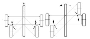
Fig. 7. Independently pivoting reaction wheel configuration. Two main drive wheels mounted at the ends of independently actuated arms produce hopping and/or stabilization motion via a combination of symmetric and antisymmetric rotation. Parallelogram linkages within each arm preserve the relative orientation of the wheels, so as to properly align the wheels for roving, and to minimize coupling of the pitch/roll/yaw axis dynamics.
