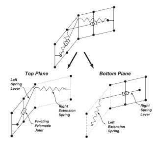
Fig. 8. The suspension mechanism consists of two symmetric halves that are mounted in separate planes to prevent collisions.
