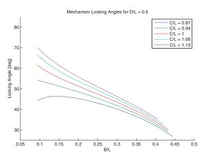
Fig. 16. The arm mechanism latching angle is a function of the linkage lengths B, C, and D. It is most sensitive spring bar length, C, particularly for small B and D.
