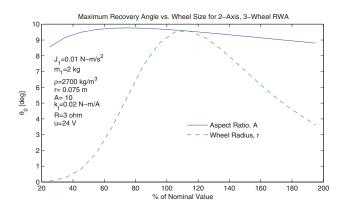
Fig. 6. Maximum roll axis recovery angle for a generic H-pattern RWA (fig. 5), as a function of: wheel radius (dashed), and wheel thickness/aspect ratio (solid). The applied torque,  $\tau = \frac{k_t}{R} \left( u - k_t \omega \right)$ , where  $\omega$  is the reaction wheel angular velocity, and u is a step voltage input.
