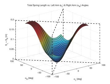
Fig. 13. Total spring length as a function of left arm angle  $(\alpha_L)$ , and right arm angle  $(\alpha_R)$ .  $\frac{B}{L} = \frac{B_2}{L} = 0.125$ ,  $\frac{C}{L} = 1.094$ ,  $\frac{D}{L} = 0.438$
