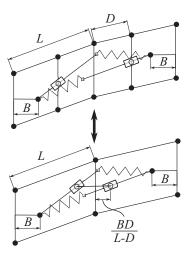
Fig. 12. Two mechanism realizations with equivalent kinematics.
