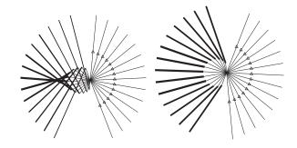
Fig. 11. Lever (solid), fulcrum (triangle), and spring (thick solid) positions throughout the nominal range of symmetric (left) and antisymmetric (right) motion, for bottom linkage plane.
