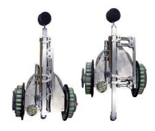
Fig. 2. Three-wheeled hopping robot, "iHop v.2" prototype. During hopping maneuvers, a reaction wheel centrally-housed within the main body stabilizes about the roll axis, and the two drive wheels stabilize about the pitch axis. A dual four bar hopping mechanism creates linear leg motion with a torque/force relationship favorable for DC motor actuation, and stores hopping energy during roving by latching into a fully-tensioned state.
