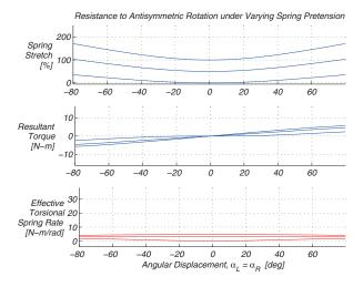
Fig. 15. Total displacement, torsional resistance, and stiffness for purely antisymmetric (balancing) motion. The resistance profile becomes more linear as spring pretension is added, resembling a conventional torsional spring.
