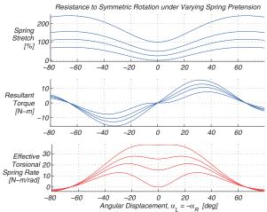
Fig. 14. Total displacement, torsional resistance, and stiffness for purely symmetric (hopping) motion. Self-latching occurs as the torsional resistance crosses zero, at  $\alpha = +/-65^{\circ}$ . Added spring pretension significantly stiffens symmetric motion about the rest position.
