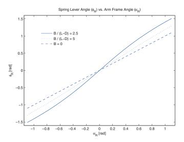
Fig. 10. The relationship between arm angle,  $\alpha$ , and lever angle,  $\phi$  becomes increasingly nonlinear as the spring lever attachment is offset inwards from the arm frame.
