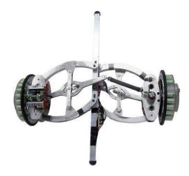
Fig. 17. "iHop v.3" prototype featuring independently actuated arms suspended via two spring-coupled linkages mirrored about the vertical axis.
