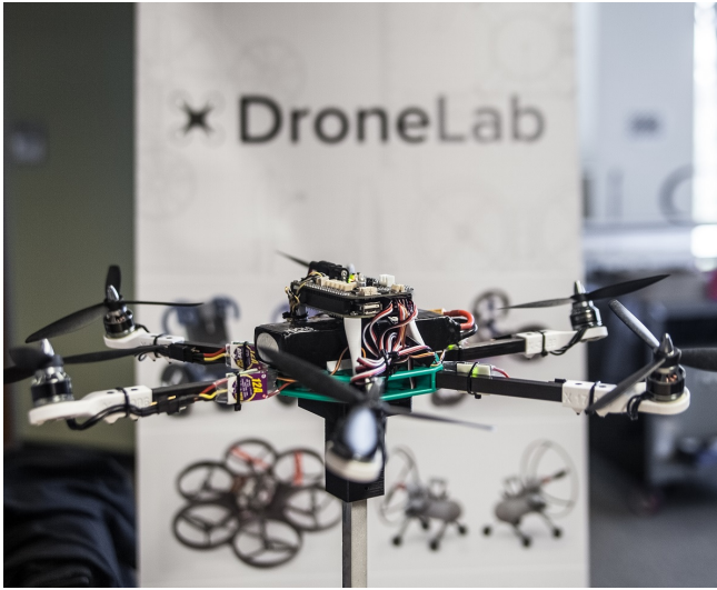
Figure 8. The thrust testing stand with optimized rotor angles
