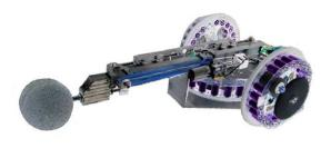
Fig. 2. Reconfigurable wheeled rover with hopping capabilities.
