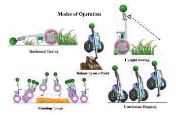
Fig. 1. Reconfigurable hopping rover capabilities. Note that the transition between horizontal and upright roving modes is achieved via a control sequence solved for using an adjoint-based optimization on the non-smooth rover dynamics [1]
