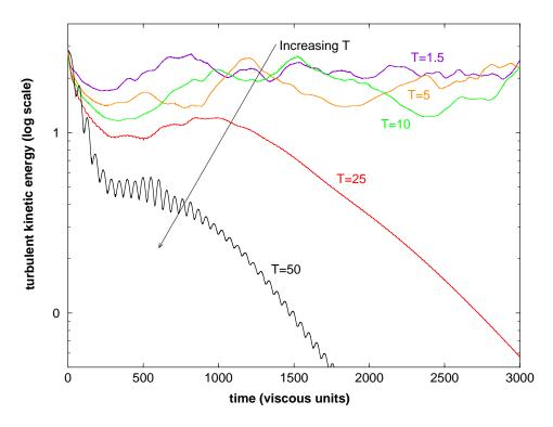
FIGURE 3. Time Evolution of the turbulent kinetic energy for different values of  $\tau$  (denoted T in the figure).
