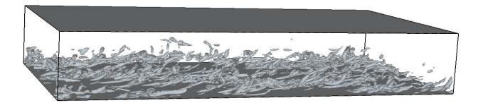
FIGURE 1. Coherent structures of a turbulent flow at  $Re_{\tau} = 180$ .
