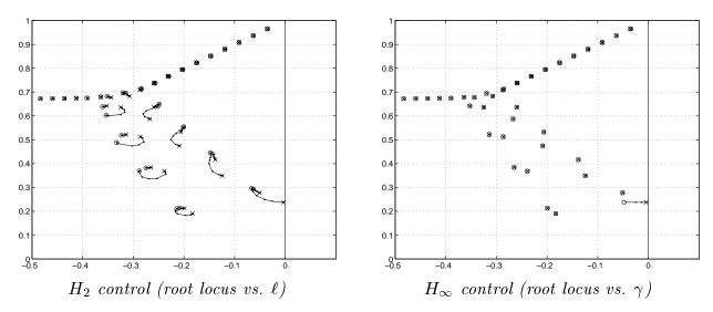
FIGURE 4. Movement of closed-loop eigenvalues versus control parameters  $\ell$  and  $\gamma$  for  $H_2$  (optimal) and  $H_\infty$  (robust) controllers applied to the Orr-Sommerfeld equation for  $Re=10,000,\,k_x=1,\,k_z=0$  using blowing/suction as the control variable.
