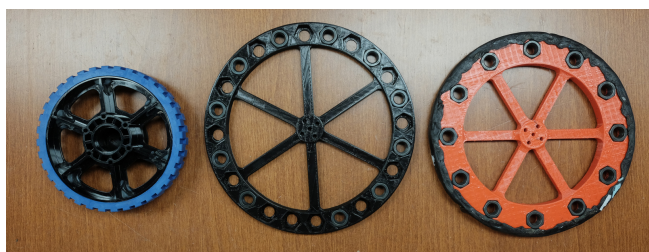
Fig. 10: Wheels tested (from left to right): off-the-shelf plastic wheel with urethane tread that was unable to achieve leg balancing. Black 3D printed wheel used for testing with slots to add mass. A red 330g wheel with rubber tread. Through optimization, we arrived at a 390g wheel.
